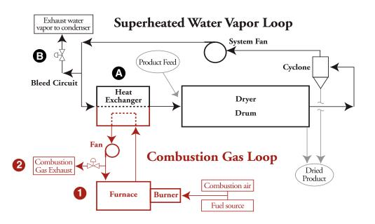
System fan creates a circulating loop of water vapor. Heat is transferred from the heat exchanger (A) to drive the evaporation of moisture from wet feed in the dryer drum. The water evaporated from the feed displaces air in the water vapor loop, creating the "airless" environment. To maintain atmospheric pressure in the dryer, a bleed circuit (B) is needed to exhaust water vapor. This water vapor can be treated with a conventional condensing system or used as a heat source for other processes.
